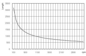
\* If rotation speed increases, ball screw may cause resonance owing to original frequency of screw axis, which causes disability of motion, so that it should be set to utilize under resonance point (risky speed).
