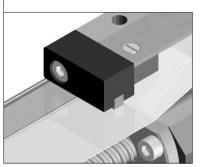
In order to prevent internal dust generation, belt is built-in and stainless steel cover is equipped.
