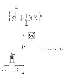
Pressure: 21 MPa (3050 PSI) Flow Rate: 16 L/min (4.2 U.S.GPM)
